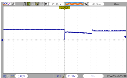
Clicker Drive Voltage (Q1 Collector)
